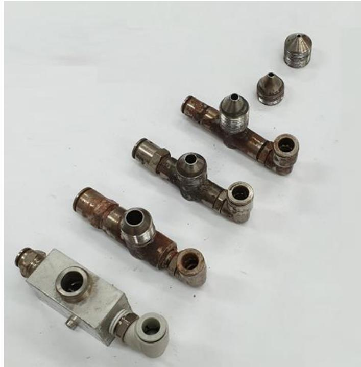
**Figure 4.8: The different underflow attachment sizes. From top to bottom: 2 mm, 3 mm, 4 mm, 6 mm, 8 mm, 10 mm internal diameter. The 3 and 2 mm parts screw onto the body of the 4 mm piece.**
