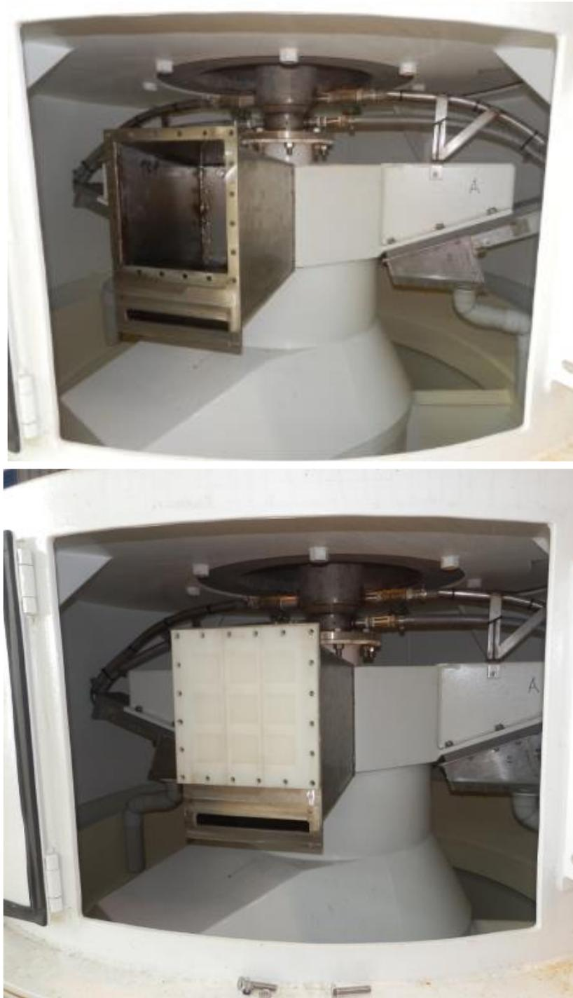
**Figure 4.1: Swinging arms of the Graviton centrifuge with an open mount (top) and with the inclined channel module in place (bottom). The centrifuge is contained within a stainless steel housing.**
