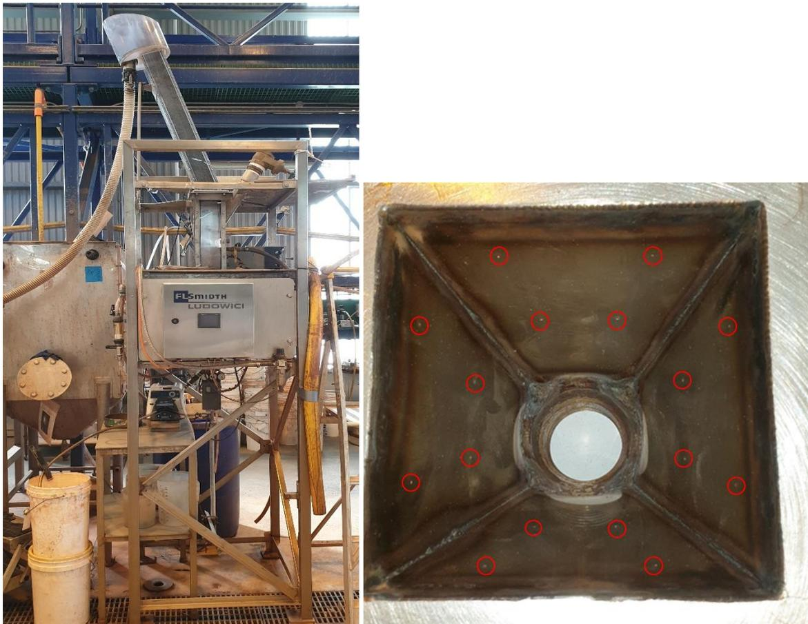
**Figure 4.20: Photo of the RC™100 (left) and the inside of the fluidisation distributor showing four holes on each face of the inverted pyramid (right).**
