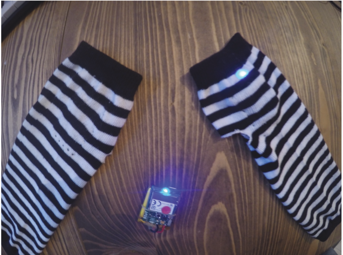
Figure 8.5: GIRD Prototype - IRCAM Riot Sensor Sewn into Gloves.
