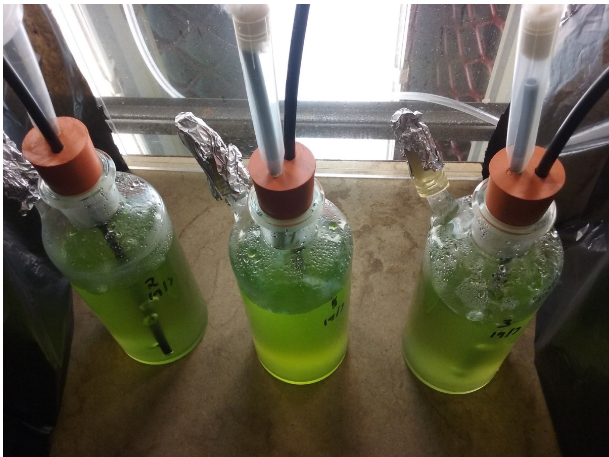
Figure 6.1 Bioreactor setup for culturing algae during the trial experiments at PSFI
