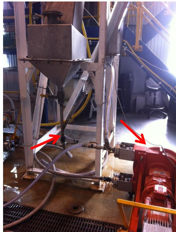
Figure I.26: The underflow exit and the underflow pump in the pilot scale runs.
