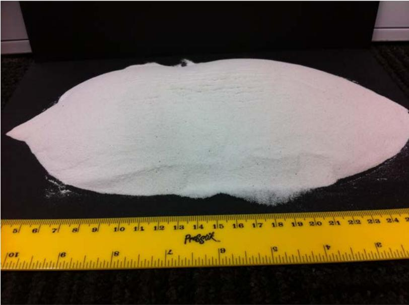
Figure I.31: Final cenospheres powder product obtained from the multi-stage IRC™ process.
