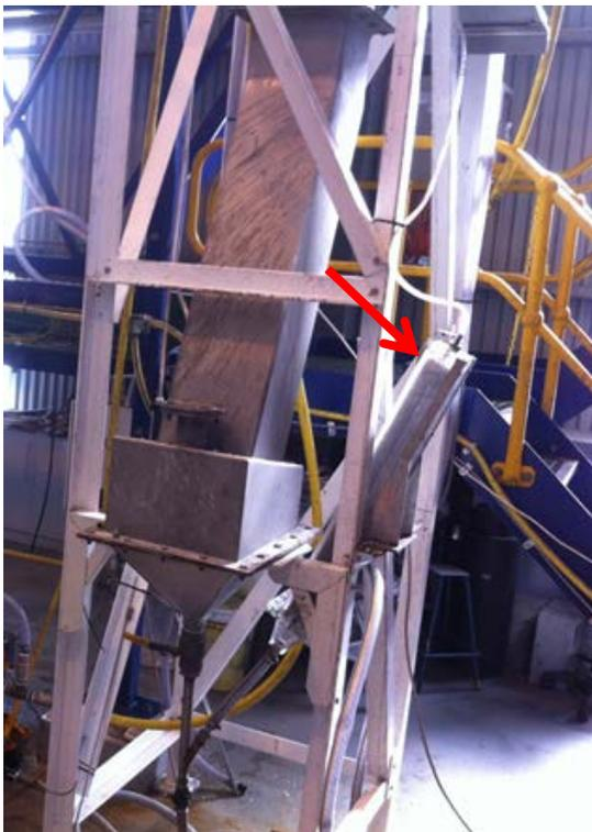
Figure I.25: The inclined channels used at the side of the pilot scale IRC™ to remove solids from underflow.
