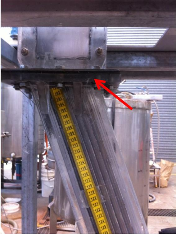
Figure I.15: The junction of inclined and vertical sections.
