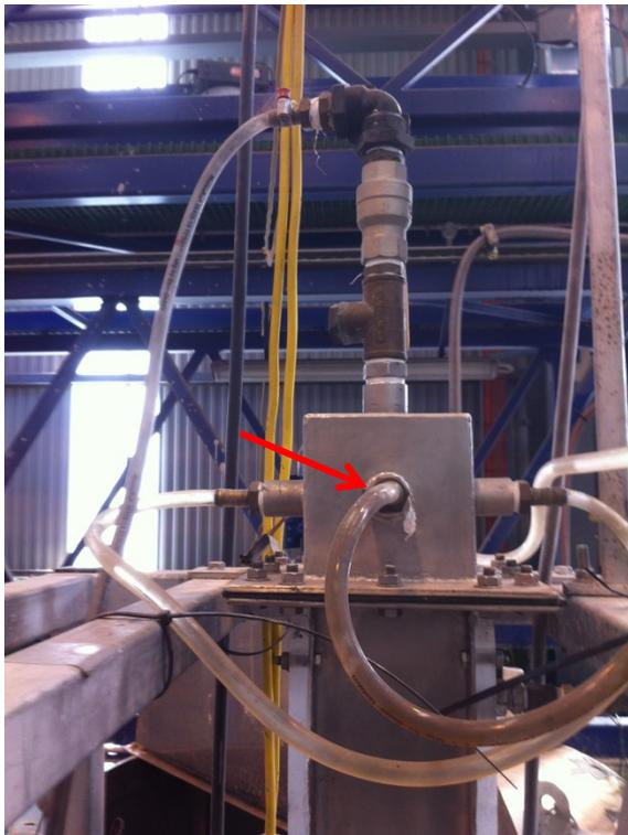
Figure I.9: Inlets to the fluidization chamber.
