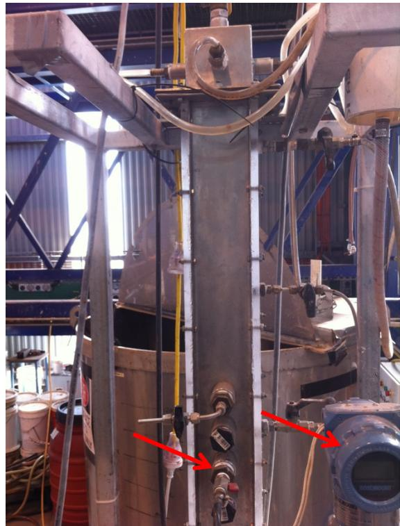
Figure I.10: Pressure transducer, feed inlet and fluidization chamber.
