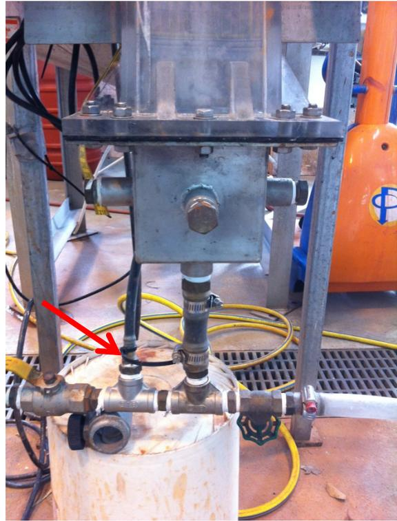
Figure I.12: The tube extended to 1 m above the IRC™ to make the system pressure balanced.
