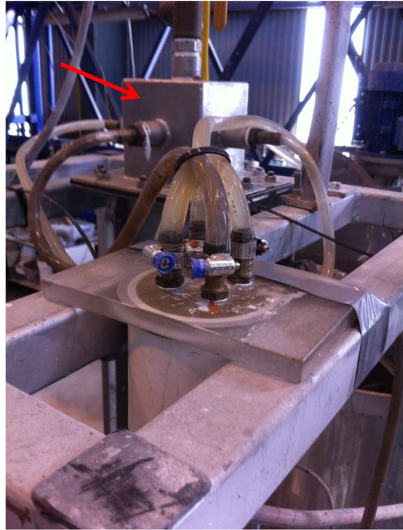
Figure I.8: Fluidization chamber in the IRC™.
