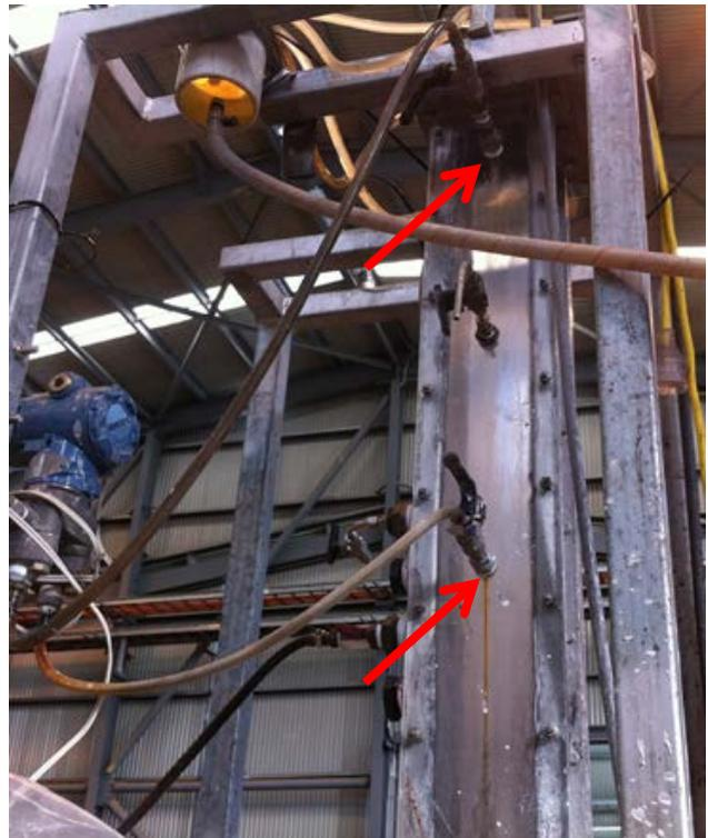
Figure I.14: The location of pressure transducer tubes.
