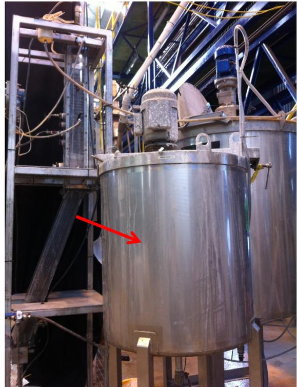
Figure I.2: Feed tank used in the lab scale runs.
