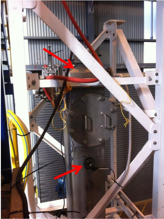
Figure I.27: Upper pressure sensor and fluidization chamber in the pilot scale IRC™.
