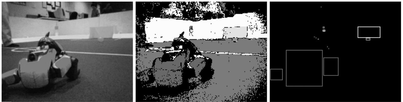
Fig. 2. Color classification process on a Sony AIBO robot. (Left) Original, unprocessed image obtained from the robot's camera. (Middle) Same image after color classification has been performed. (Right) Colored blobs that have been formed based on the color classified image. (For printing, colors have been converted into grayscale.)
