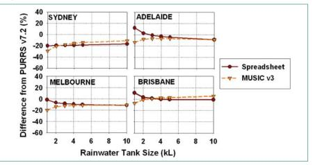
**Figure 7.** Difference in results from the use of equal rainfall durations in Spreadsheet and MUSIC when compared to PURRS.
