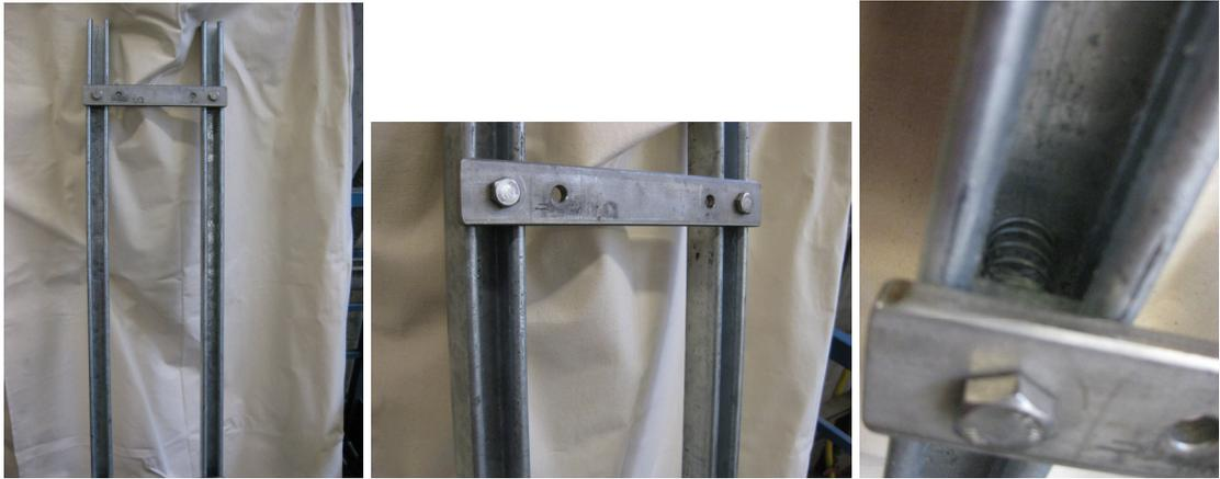
Figure 3: Photograph showing the N1000 frame and the struts used to mount the Reflux Classifier apparatus onto the frame.
