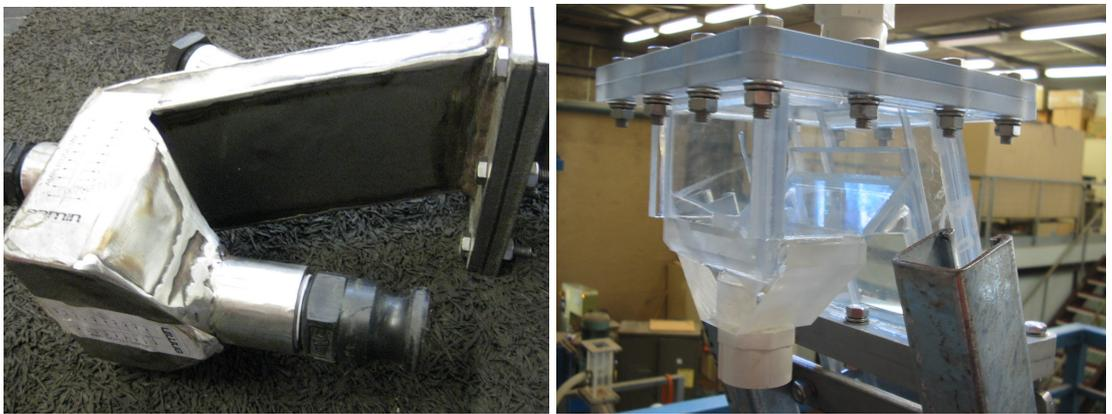
Figure 4: Photographs of the overflow arrangement showing the stainless steel that was used for the majority of experiments as well as the polycarbonate arrangement to give insight into the internals of the stainless steel.
