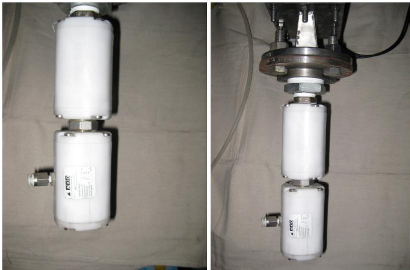
Figure 6: Showing the pinch valves below the pyramid section.
