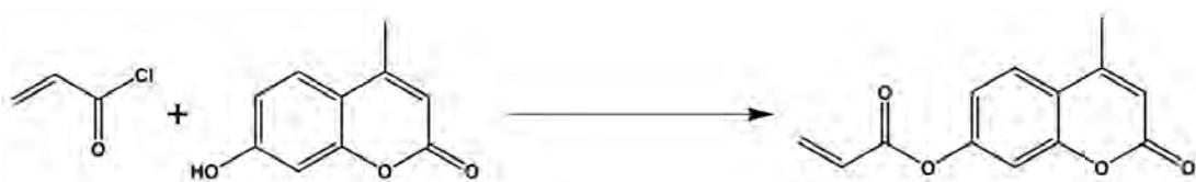
**Figure 2.2:** Synthesis of 7-hydroxy-4-methylcoumarin acrylate (HMCA).
