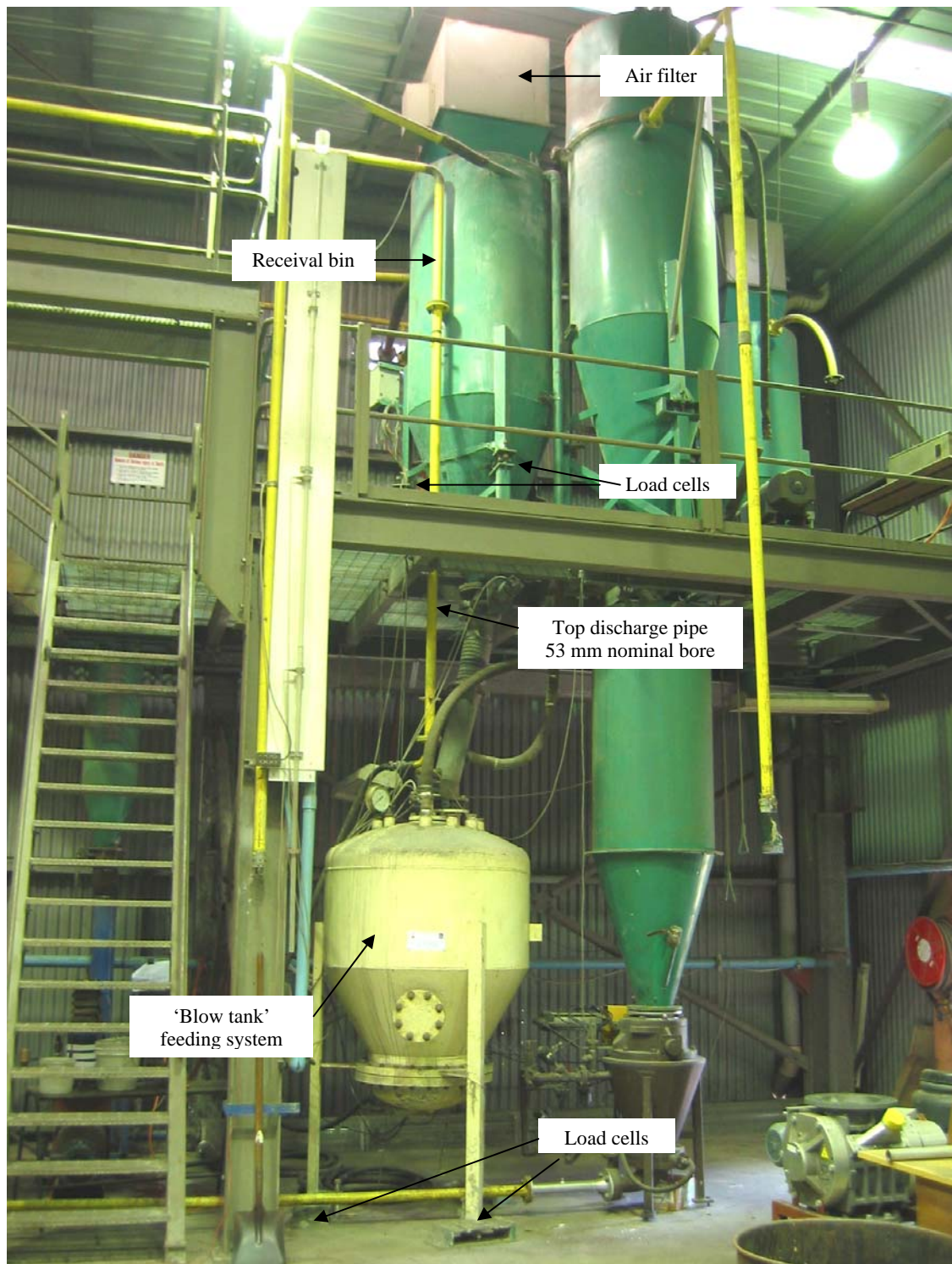
Figure 31, pneumatic conveying feeding and receival systems used in the conveying trials
