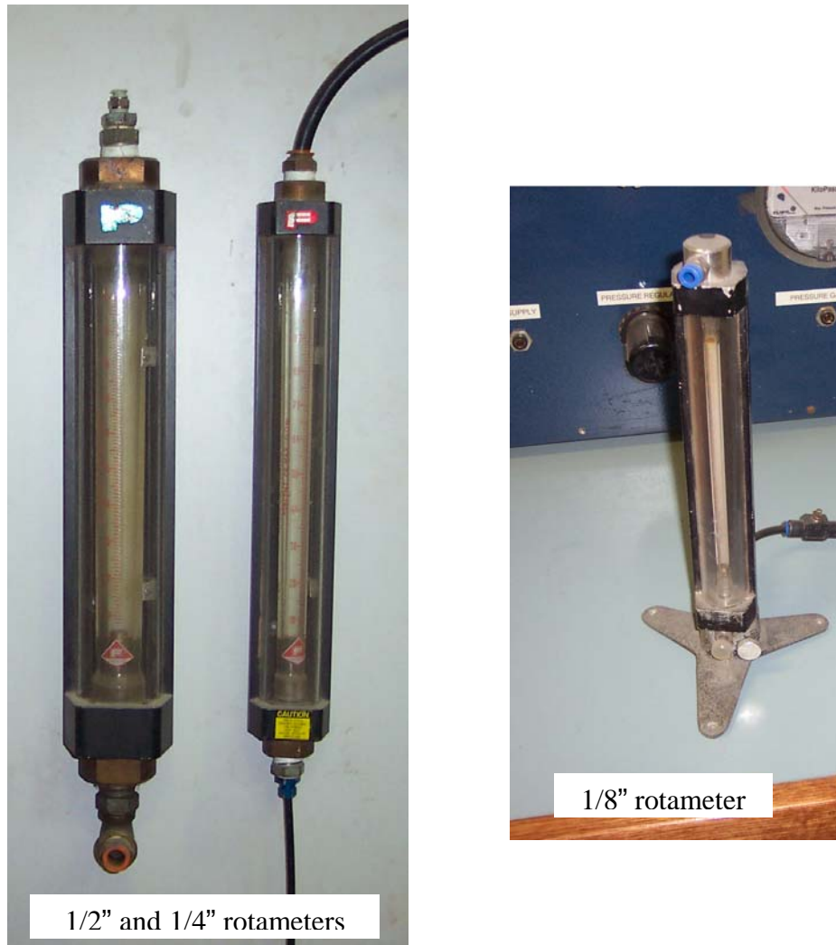
Figure 24, rotameters used in fluidisation tests
