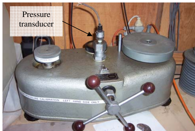
Figure 33, picture of the Barnett ‘dead weight’ tester used for calibrating the pressure transducers and calibration plot
