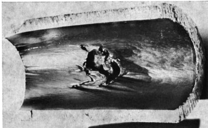
Figure 2-2: The wear produced by abrasive and erosive wear at the same time [7].
