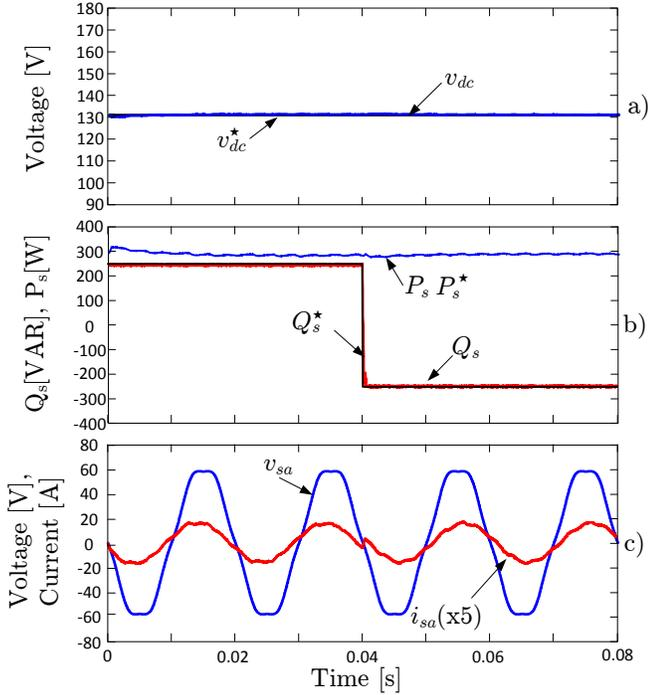
Figure 7. Performance of the MPC algorithm presented – Simulation: step in the reactive power reference  $Q_s^*$ .
