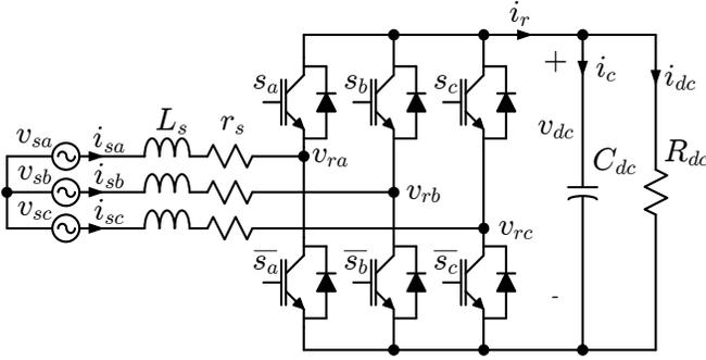
Figure 1. Active front-end rectifier with floating neutral point
